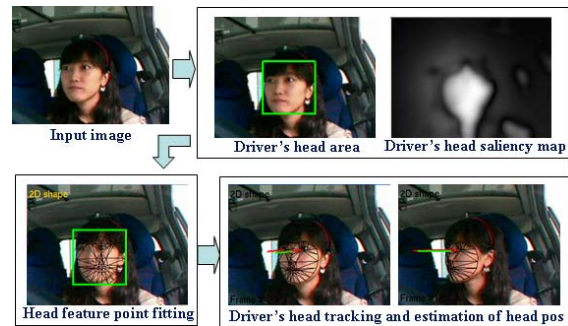
Fig. 5. The procedure of active appearance model for tracking driver's head and estimating driver's head pose.
